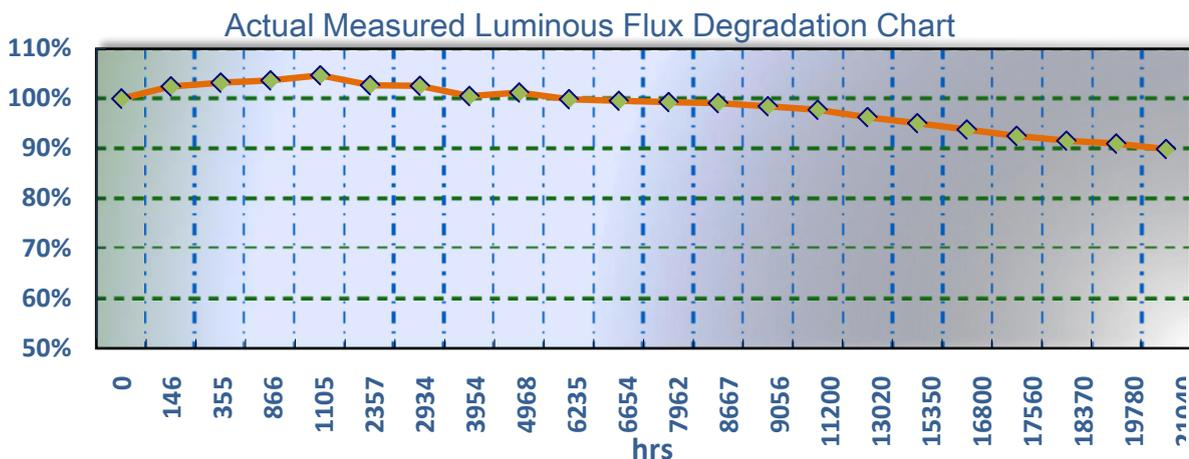
Remarks: This chart shows the actual testing data of many streets that exactly reflects luminous flux degradation of LED street lights in use. It is noticeable that natural environment conditions such as weather, temperature and so on can affect illumination intensity to some degree in actual testing. We can see that the maintaining luminous rate of our street lights is above 95% after working for 3 years without maintenance.
