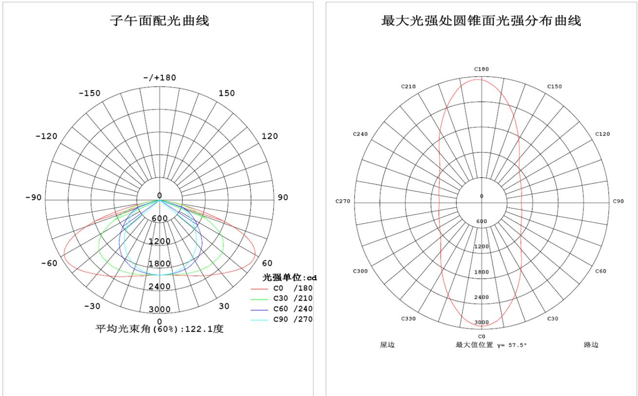
Remarks: The bat-wing light distribution forms a rectangular facula in the effective area on the road, ensuring the illumination uniformity in the longitudinal direction is above 0.5 and the total illumination uniformity on the road is above 0.4.
